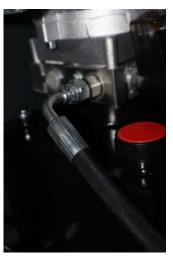
• With the hydraulic hose connected to the pump, fill the tank with hydraulic fluid.
